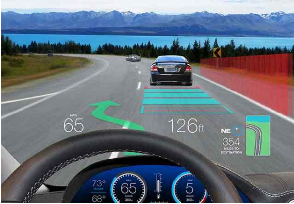
Fig. 7 Augmented Reality Head Up Display Source : Texas Instrument AR Head up display white paper, 2017
