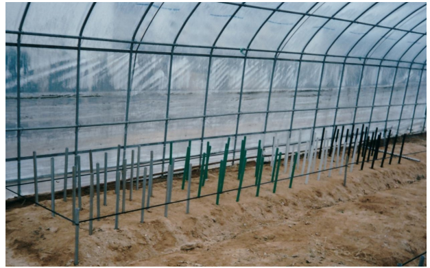
Fig. 1. Photo of corrosion protection treatment pipes buried in greenhouse.
