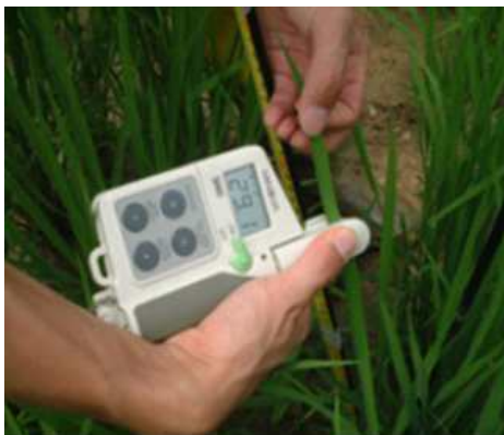
Fig. 2. Chlorophyll measurement sensor
