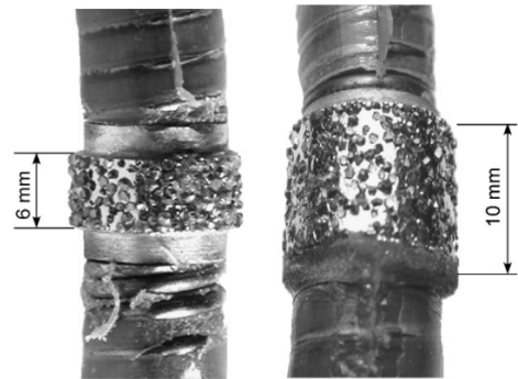
Fig. 4 Narrow (left) and standard (right) diamond beads [19]
