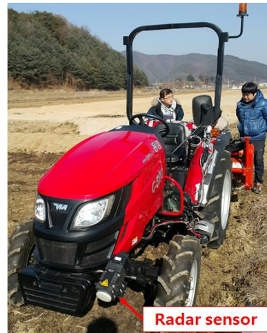
Fig. 7 Radar sensor for actual working speed measurement.
