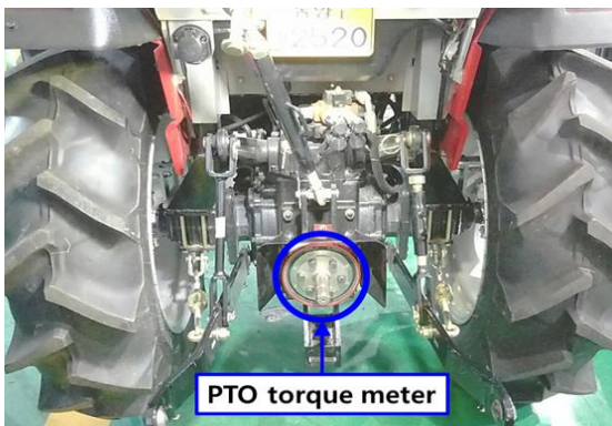
Fig. 6 A view of Torque meter mounted on the PTO shaft
