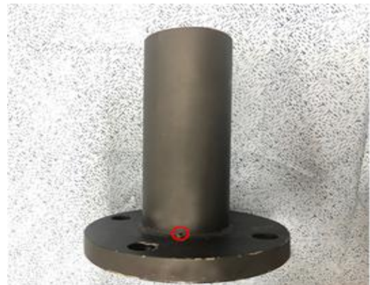
Fig. 1 Carbon steel pipe flange specimen
