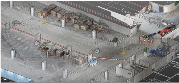
Figure 7. 3D scanning of apartment's parking building
