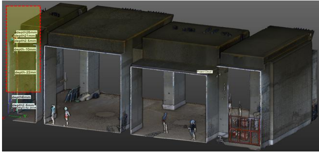
Figure 10. 3D scanning result of piloti column
