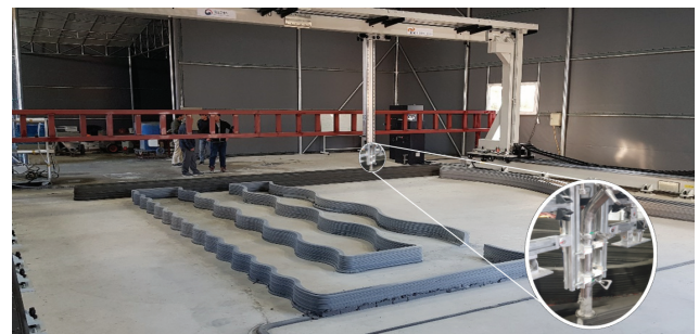
Fig. 3 3D Printer in test-bed(KICT) and Nozzle (right)
