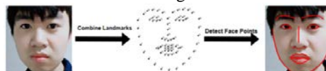
Fig. 3. Match the face profile with 68 landmarks and then correct to the center.
