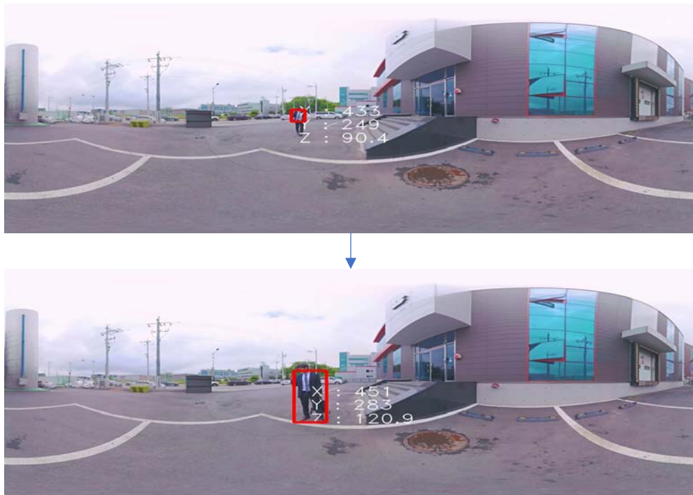
Fig. 13. The extracted 3D positions of the target object in the 360-degree drama frames
