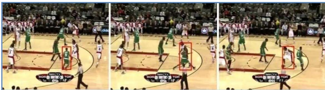
Fig. 2. A scenario of drift case in GOTURN tracker . Left : Target object with bounding box (Red) Middle : Another object occluded with the target object Right : Target changed to another object.
