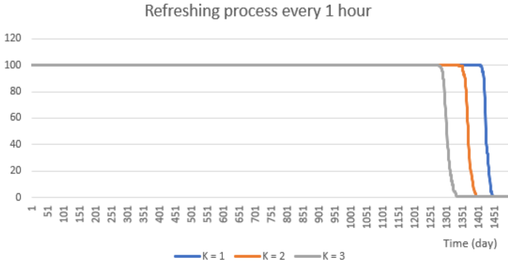
Fig. 18. The number of active nodes when K is 1, 2, and 3 with refreshing process every 60 mins
