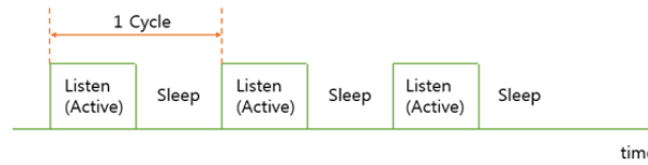
Fig. 1. Basic scheme of S-MAC with periodical listen and sleep
