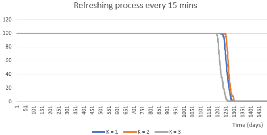
Fig. 16. The number of active nodes when K is 1, 2, and 3 with refreshing process every 15 mins
