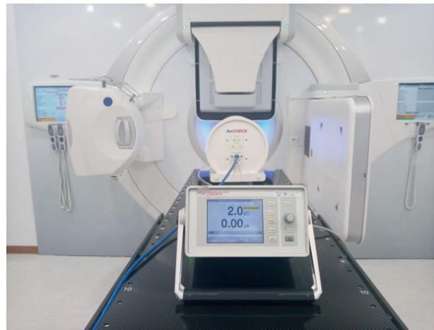
Fig. 2. Linear accelerator with phantom and ion chamber installed
