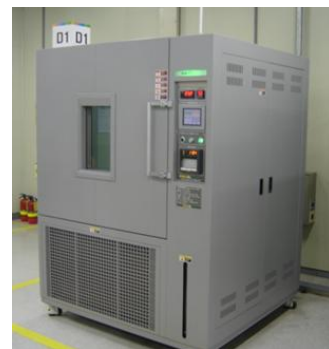
Fig. 3. A temperature controllable chamber used for high-temperature environmental test.
