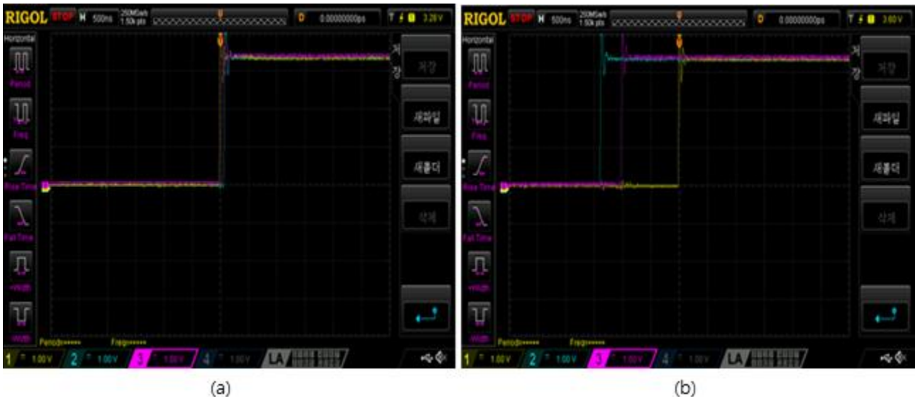
Fig. 5. Results of 1-PPS performance test over time of time synchronization error.
