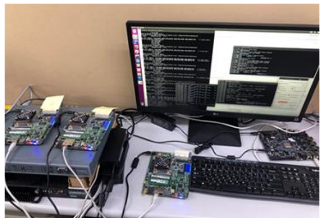
Fig. 3. Test environment of PTP time synchronized system the implemented IED platform.
