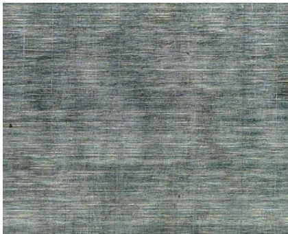
Fig. 11 Photography of tool surface after 97 th test (Ra : 0.225 \mu m, Transverse direction)
