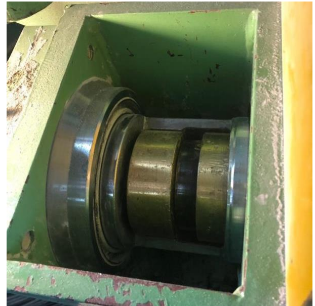
Fig. 9 2 stage die in the wire drawing apparatus
