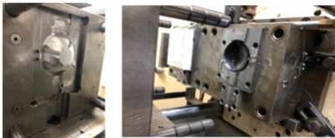
(a) Movable mold (b) Stationary mold Fig. 15 Fabricated mold for film insert molding
