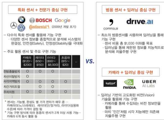
[Figure 2] Traditional method and deep learning-based method for ADAS[16]
