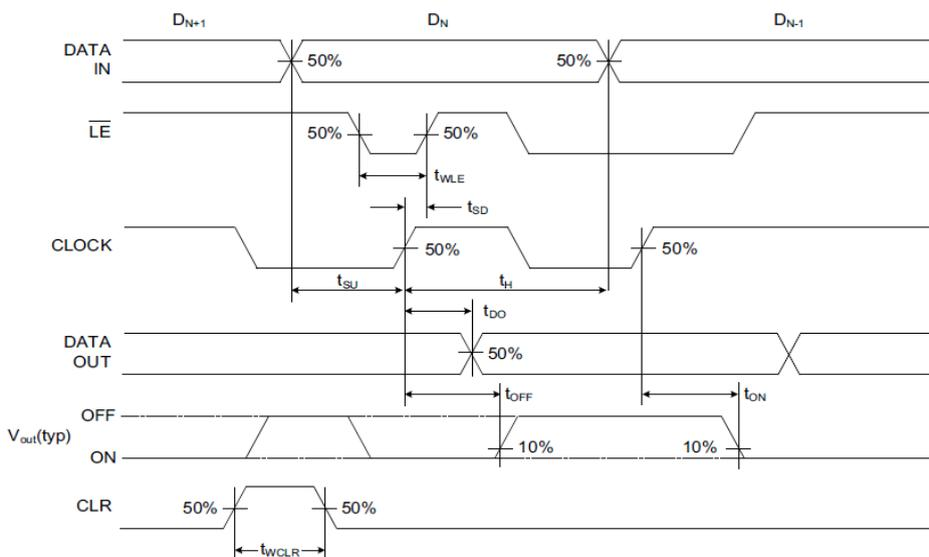
[Fig. 3] Logic Input Typical Timing Diagram
