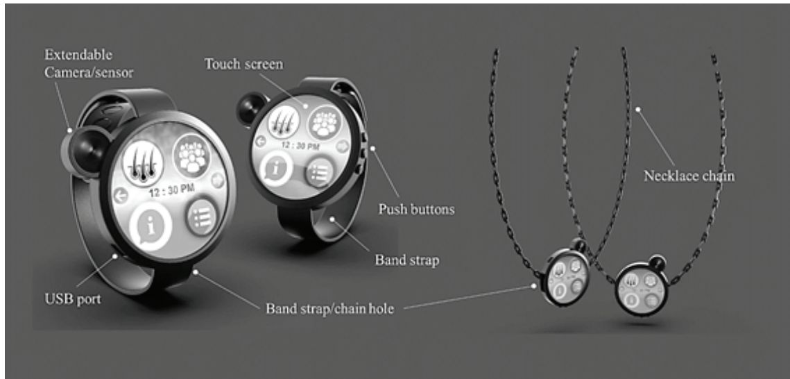
Fig. 1. 3D virtual design for hair designers (Left: bracelet/watch type with a band strap, Right: necklace type with a chain).
