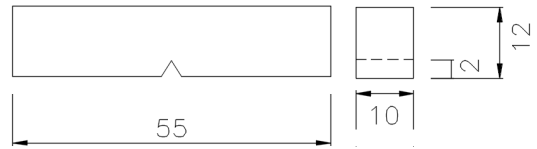
Fig. 2. Configuration of Charpy impact specimen.
