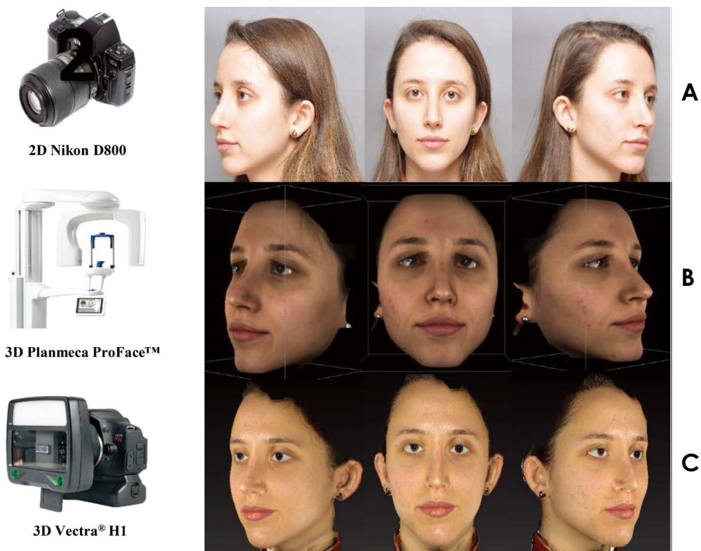
Fig. 2. Image acquisition. A. Two-dimensional camera. B. Three-dimensional laser scanner. C. Three-dimensional stereophotogrammetric device.
