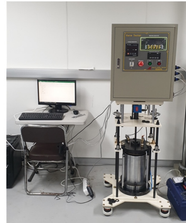
(b) Photograph of laboratory pressurized vane test apparatus
