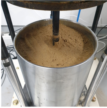
Fig. 5. Preparation of foam-soil mixture before test
