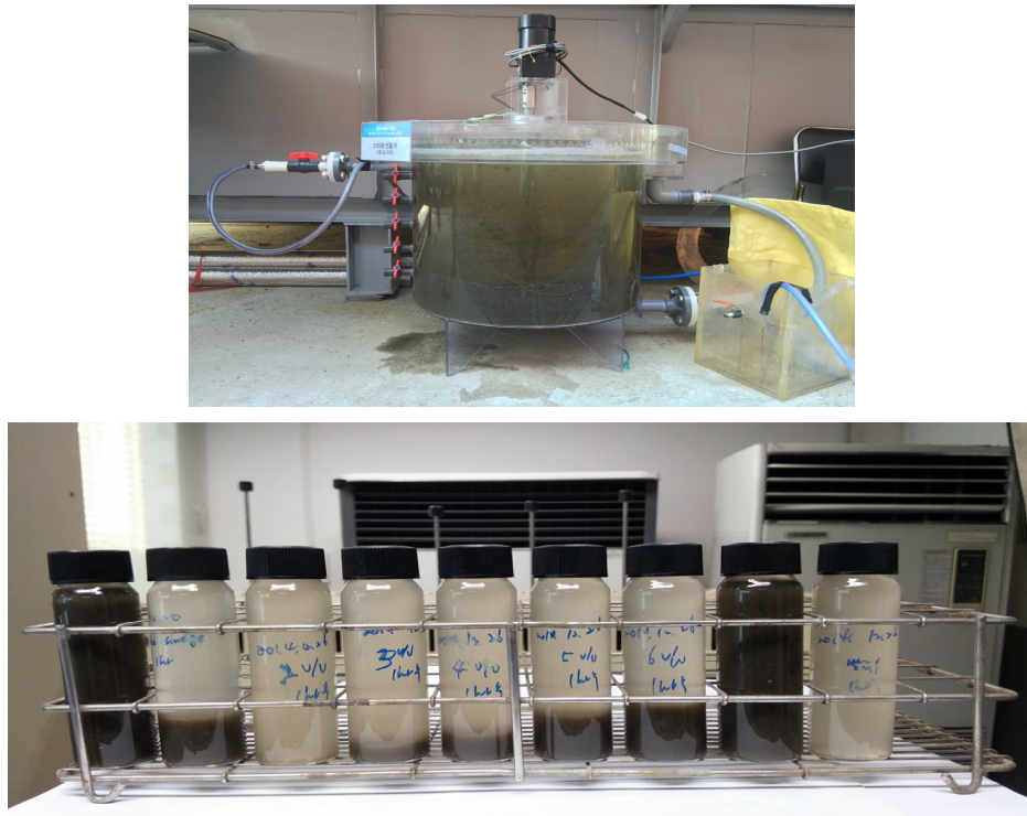
Fig. 3. Changes in sludge concentration with the changing heights of a settling tank.
