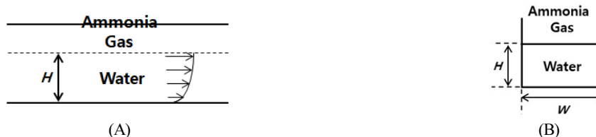
Fig. 1. Water flow exposed to ammonia gas(A: Side view of the flow, B: Cross-sectional view of the flow. Rightward arrows indicate the direction of the flow.)
