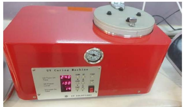
**Figure 2.** V cure post-curing machine.
