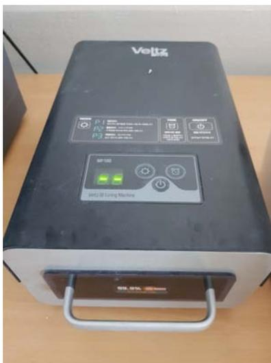
**Figure 1.** MP100 post-curing machine.
