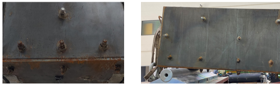
(a) Side plate and bottom plate (b) Sliding between steel and concrete <Fig. 6> Test result of steel plate
