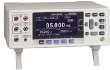
Fig. 4 Low resistance meter (HIOKI RM3544)
