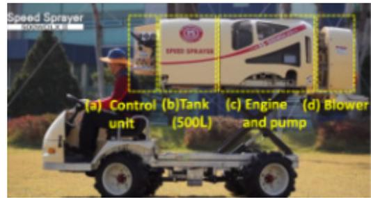
Fig. 1 General speed sprayer used in orchards
