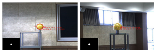
Fig. 3 Target detection using color and shape
