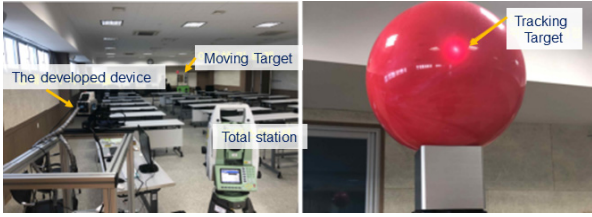
Fig. 8 Positioning test conducted indoors
