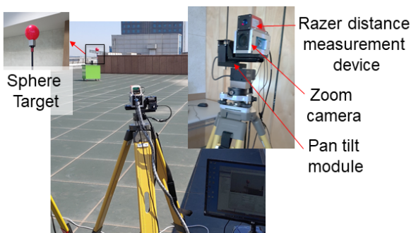
Fig. 2 Configuration of relative position measuring device
