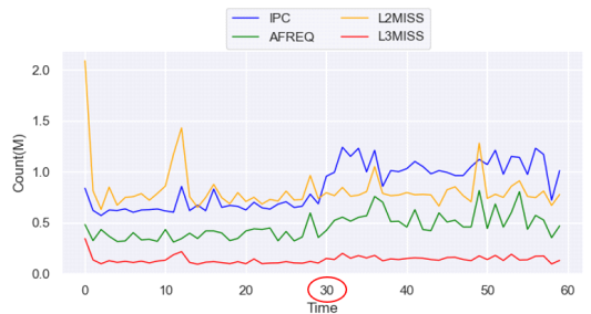
Fig. 7. IPC, AFREQ, L2MISS, L3MISS count values when trying key attack on AES
