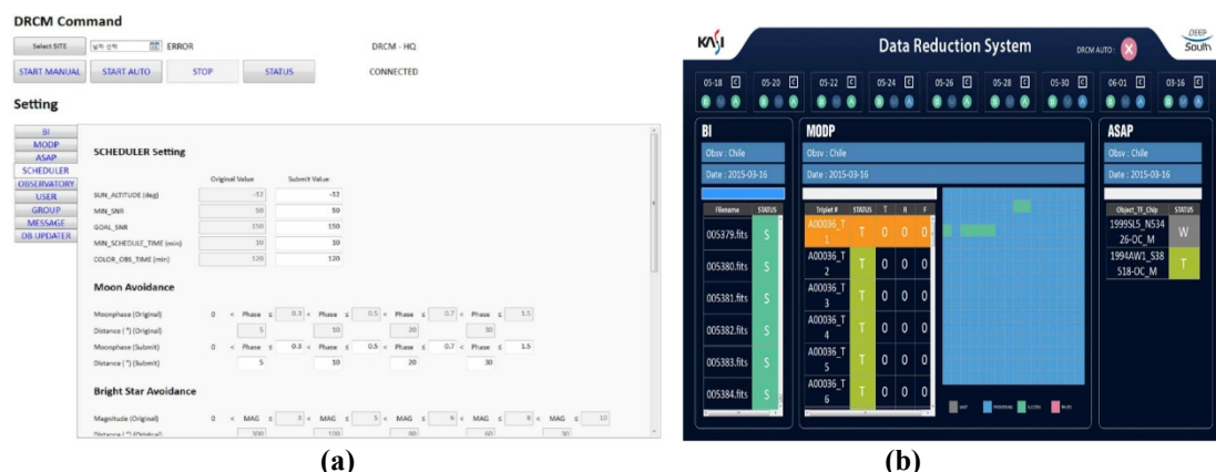
Figure 8. KMTNet controller GUIs for monitoring, searching and analyzing Near-Earth Objects (NEOs). (a) Telescope controller and (b) Data reduction
