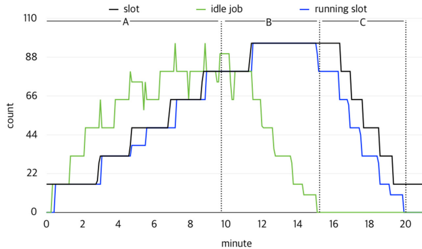
Figure 5. Dynamic resource allocation according to the number of idle jobs and running slots
