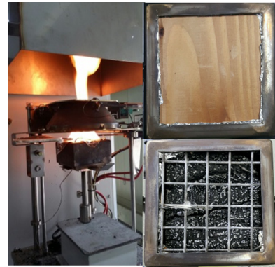
Figure 1. ISO 5660-1 Cone calorimeter experiment.
