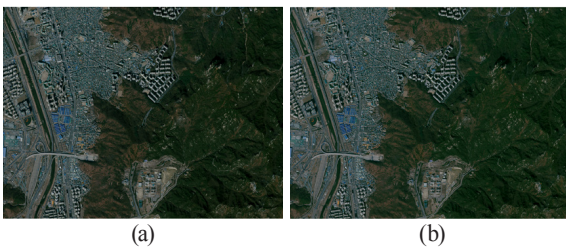
Fig. 5. Comparison with the results of relative radiometric normalization for Site 2: (a) global histogram matching, (b) proposed method
