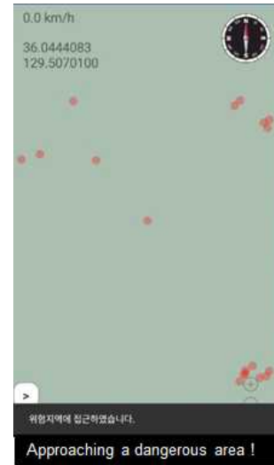
Fig. 12 Notification and voice message for dangerous area
