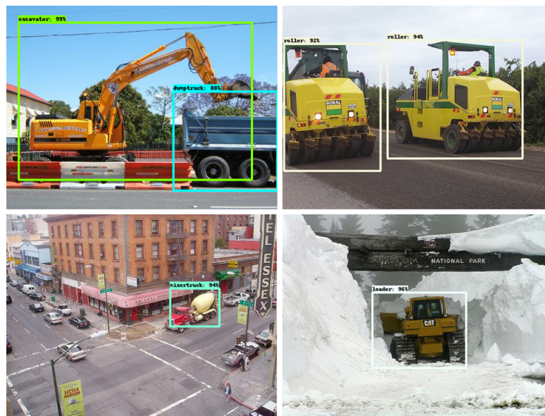
Fig. 3. Examples of Construction Object Detection
