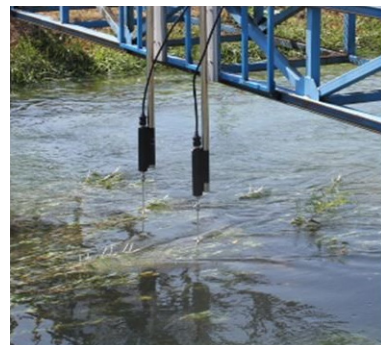
Fig. 5. Flow Measurements with ADV
