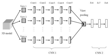
Fig. 1. Architecture of MVCNN model.
