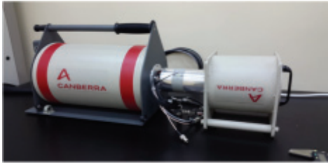
Fig. 1. Gamm-ray measurement spectrometer system (HPGe detector) of gamma-ray from the nat Pb sample.
