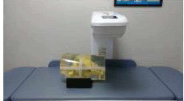
Fig. 2. Human phantom rotation BMD measurement setup.
