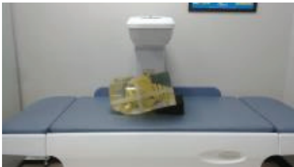
Fig. 4. Human phantom was inclined from 0 to 20 degrees setup.
