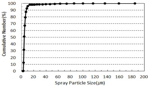
Fig. 5. Cumulative number(%) according to spray particle size in the range of Ra = 12.70~22.84 $\mu\text{m}$  when BLDC sirocco fan revolution is 5,600rpm and salt water supply rate is 19.70mL/min.
