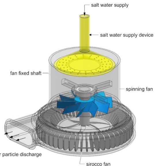
Fig. 1. Rotary mist spraying device.
