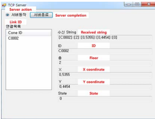
Fig. 11. IoT Cone mode change message reception screen on safety management server
