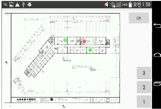
Fig. 10. IoT Cone setting UI for the danger zone
