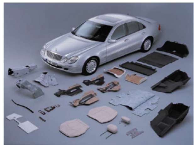
Figure 21. Mercedes-Benz, bio-composite materials applied to ‘Mercedes Class E’ [86].
