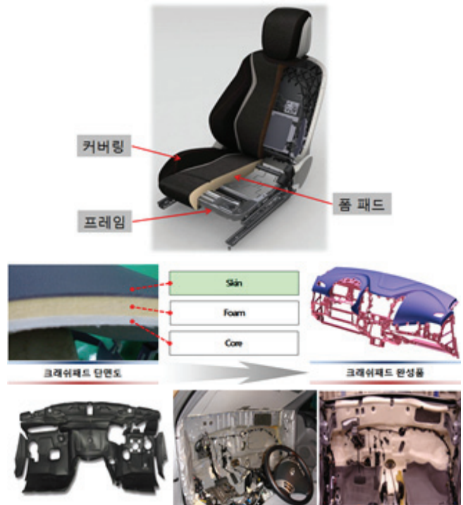
Figure 20. Polyurethane foam applications (car seats, crash pads, dash iso pads) [5].
