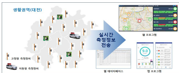
Fig. 1. Composition Diagram of Environmental Safety Real-Time Monitoring System by Living Area.
