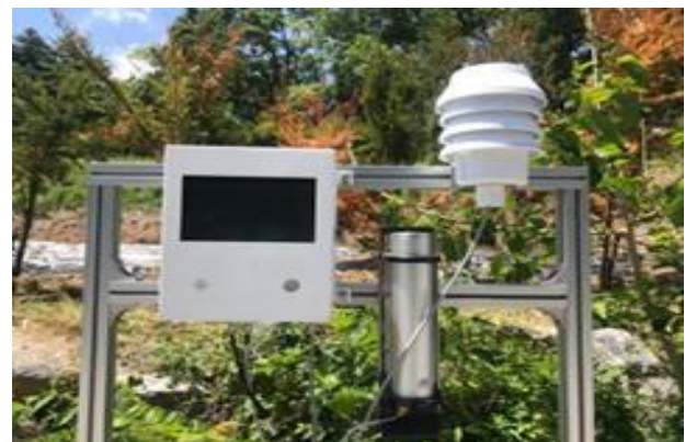
Fig. 3. Hardware Image of Fixed Measuring Equipment.
