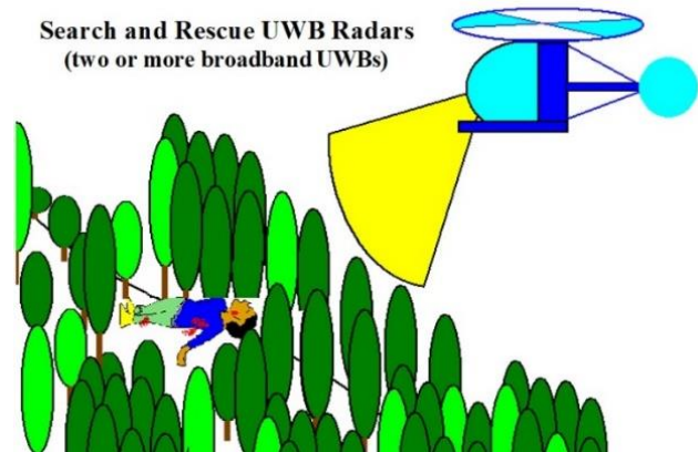
Fig. 18. UWB radar for location people lost in the woods.
