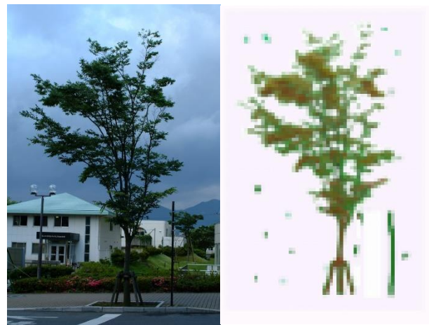
Fig. 17. Result of field test by the foliage scanner, Zelkova.
