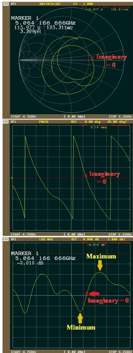
Fig. 14. Approximation of scalar value of receiving power travelling through free space. The upper part is the Smith chart, the middle part is the phase (the Y axis represents the imaginary component and X axis frequency), the lower part is the scalar value of received power, while X axis is frequency. The red marks are the phase = j0 .
