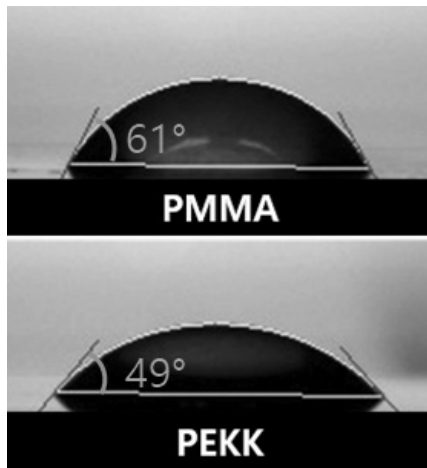
Fig. 4. Result of water contact angles of experimental groups measured by surface electrooptics
