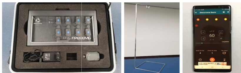
Figure 1. Methods of measurement: (a) electromyogram, (b) target bar, and (c) metronome beats
