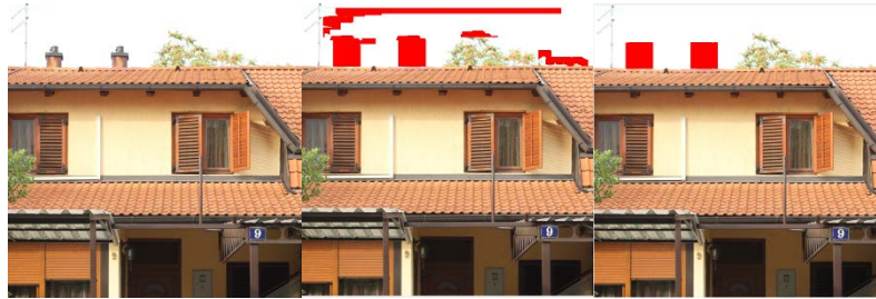
Fig. 2. Copy-move forgery detection result: (left) tampered image, (middle) initial result on detection with false positive and (right) result after false positive removal.
