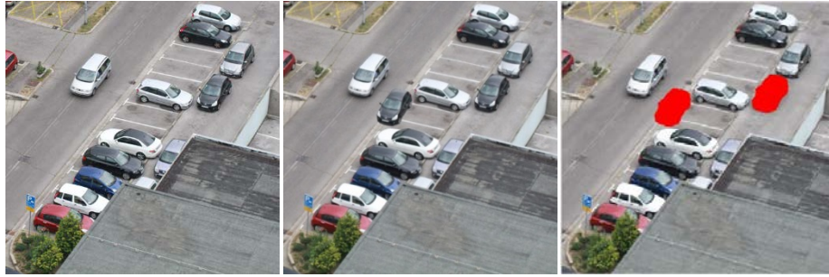
Fig. 4. Forgery detection in images with multiple copy-move tampering: (left) original image, (middle) tampered image and (right) detection result. The first, second and third rows represent blurring, brightness and colour reduction attacks, respectively.
