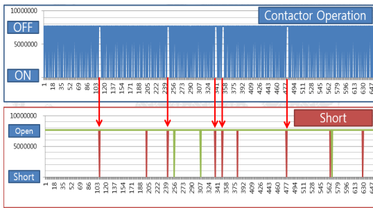
Fig. 8. Contactor Short Test Result
