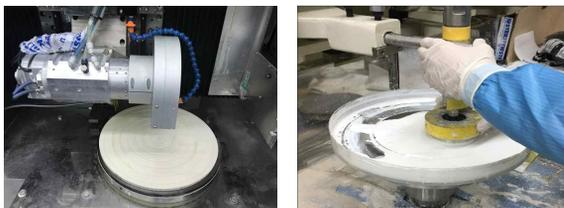
(a) Grinding Process (b) Polishing Process
